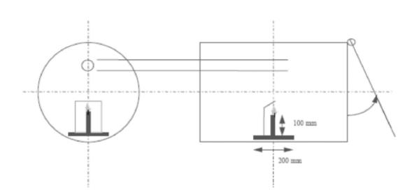
(f) the drum is laid on the ground or on a support at a spot where the temperature is between 15 °C and 25 °C; the product to be tested will be sprayed within the drum of roughly 200 dm<sup>3</sup> in which there will be a source of ignition.
